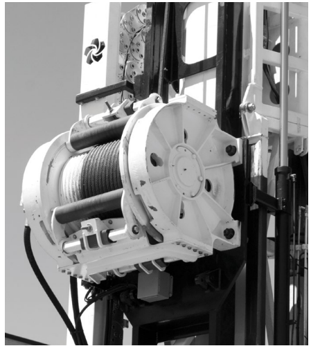
The mainline hoist (above) uses a hoisting plug (below) to pull multiple rods from the borehole at once. The hoisting plug is mounted to the free end of the top rod, replacing the water swivel.
