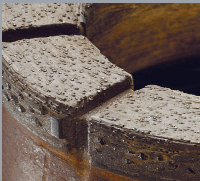
Ideal bit wear with exposed diamonds.
