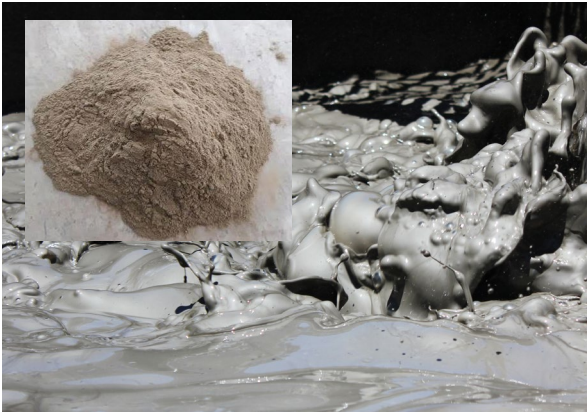
Adding Sodium Bentonite to drilling fluids will create a mud slurry.
